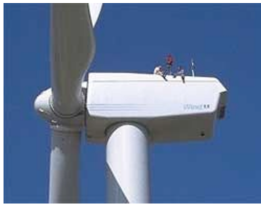
A 200 ft (65m), 1.5MW wind turbine at the Trent Mesa Wind farm in Texas
